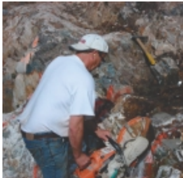
Phase One cutting channel samples in October, 2007
